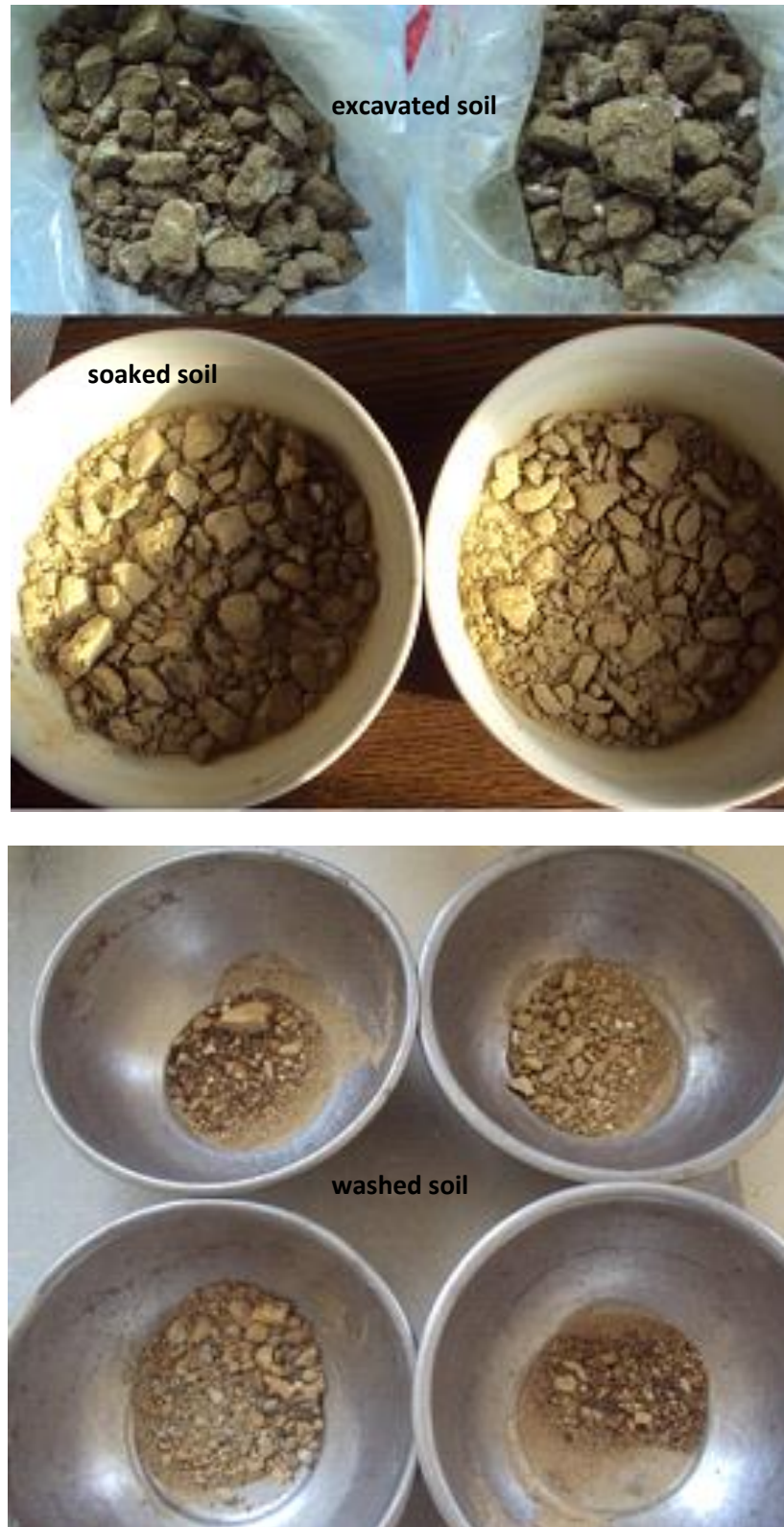
Figure 5. Breakdown of weathered rock with soaking and remaining part after washing
